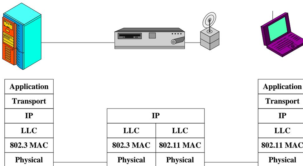
Figure 1: Router and protocol stack.
