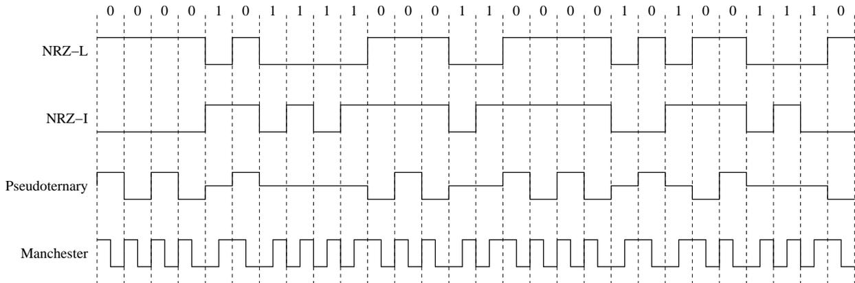
Figure 4: Example encoding of 12345678 using digital encoding techniques.
