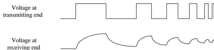
Figure 3: Attenuation of a digital signal.
