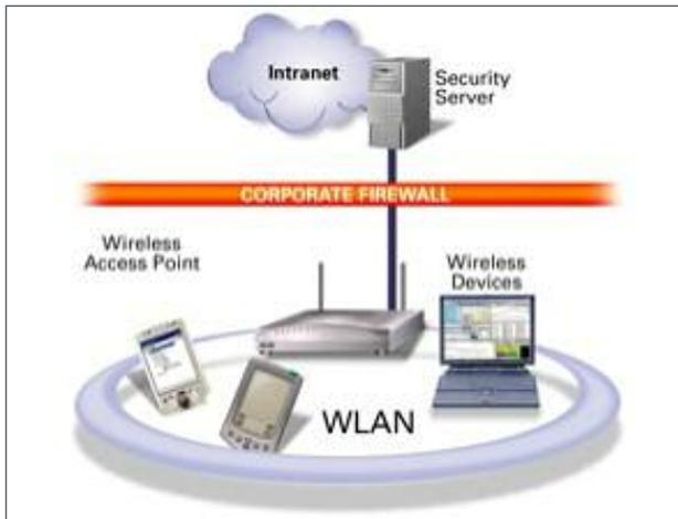
**Figure 2: A Typical WLAN Environment**
